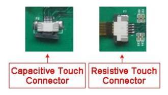
Figure 671: Capacitive or Resistive Touch Connector
