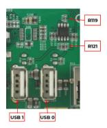
Figure 673: USB HOST Connectors (embedded/enclosed PC version)
