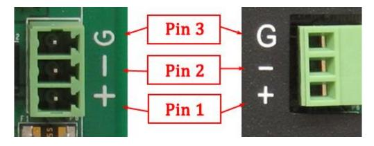
Figure 670: Power Input (embedded/enclosed version)
