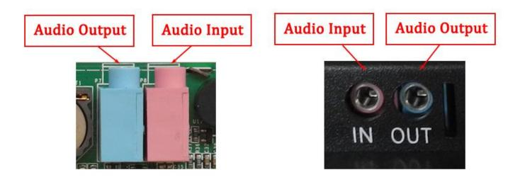
Figure 677: Audio I/O (embedded/enclosed PC version)
