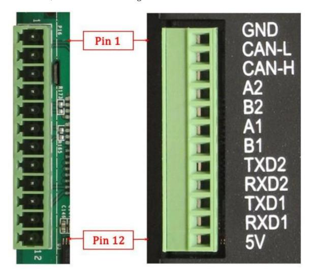
**Figure 672:** Relation between serial pins on embedded vs. enclosed version of the **EPC/PPC-A8-050-C**Industrial PC
