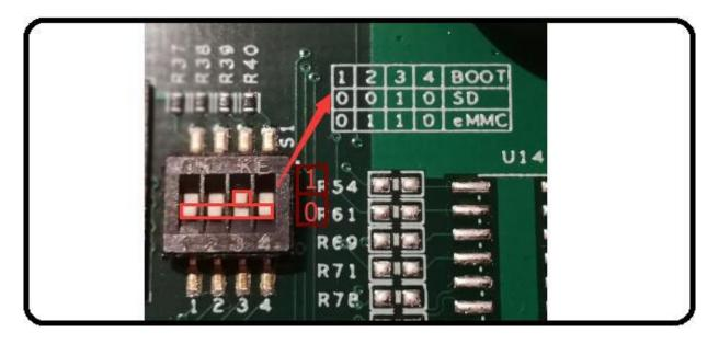
Figure 817: Boot Mode Setup
