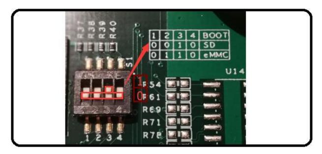
Figure 794: Boot Mode Setup
