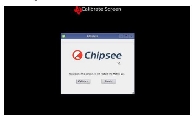
Figure 796: Resistive touch screen calibration app
