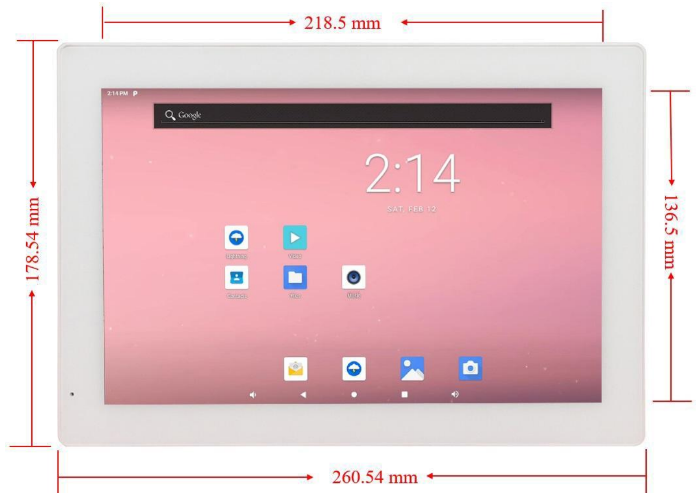
Figure 847: Front Panel Dimension Technical Drawing
