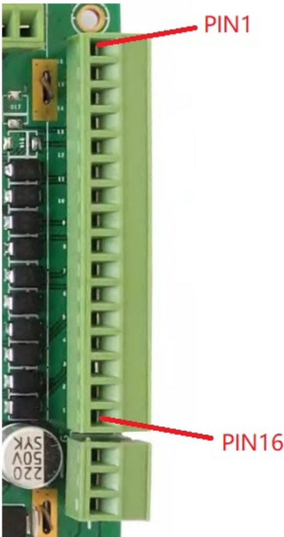
Figure 406: Relation between serial pins on embedded vs. enclosed version
