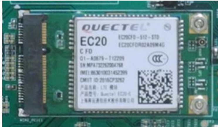
Figure 522: mini-PCle Connector & 4G Module
