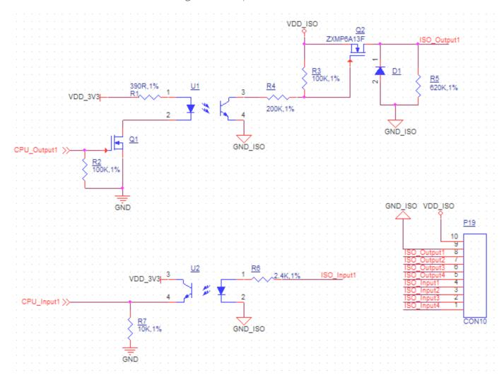
Isolated GPIO reduced schematic
