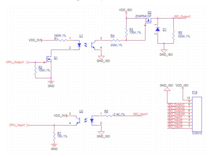
Isolated GPIO reduced schematic
