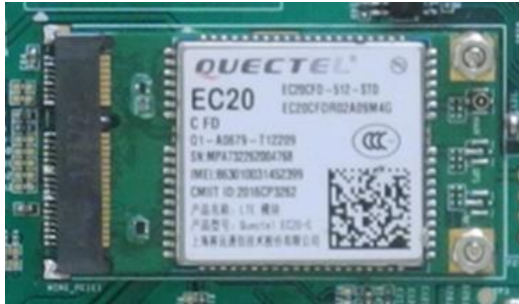
Figure 471: mini-PCle Connector & 4G Module
