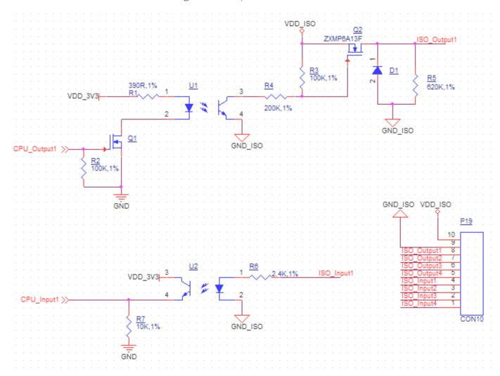
Isolated GPIO reduced schematic
