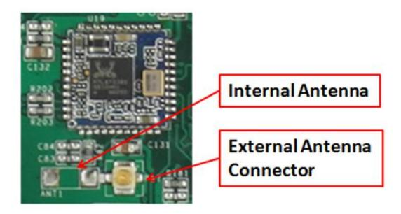
Figure 504: RTL8273 WiFi/BT Module
