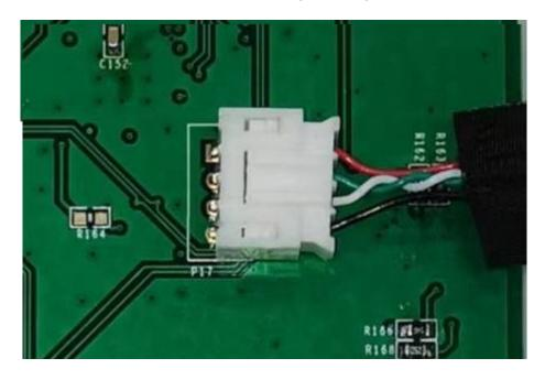
Figure 503: Capacitive Touch Screen Connector
