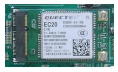
Figure 505: mini-PCIe Connector & 4G Module
