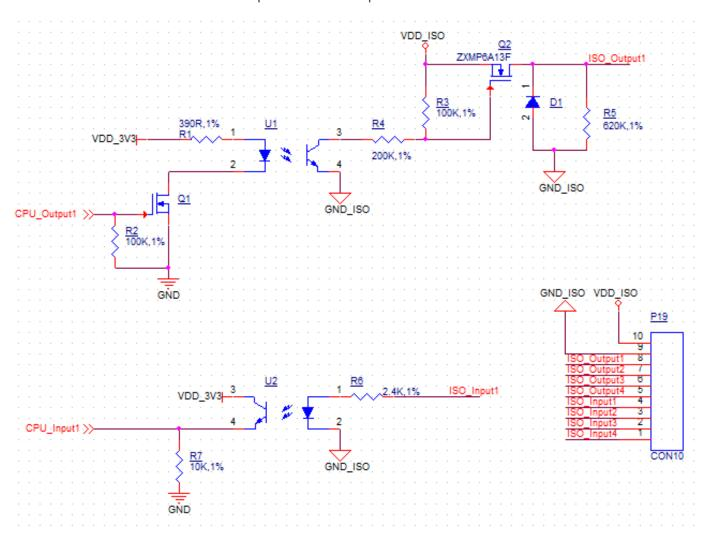
Isolated GPIO reduced schematic
