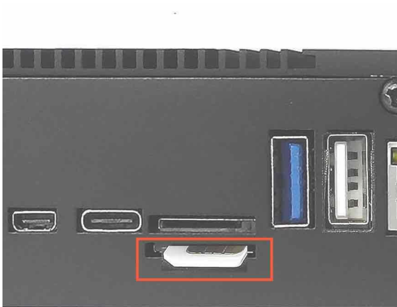
Figure 666: SIM Card Holder & 4G Antenna
