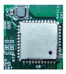
Figure 607: RTL8821CS WiFi/BT Module
