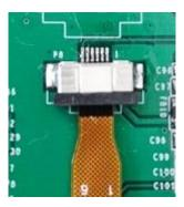
Figure 606: Capacitive Touch Screen Connector
