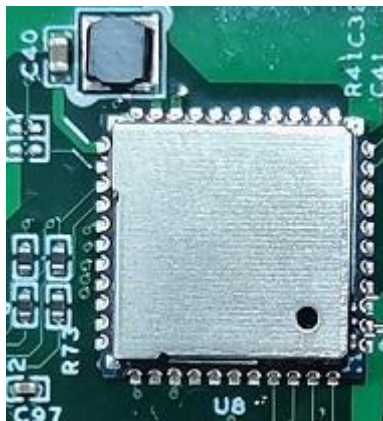
Figure 614: RTL8821CS WiFi/BT Module
