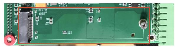
*M.2 2280 Slot for PCI-E 3.0 x 2 NVME SSD*
