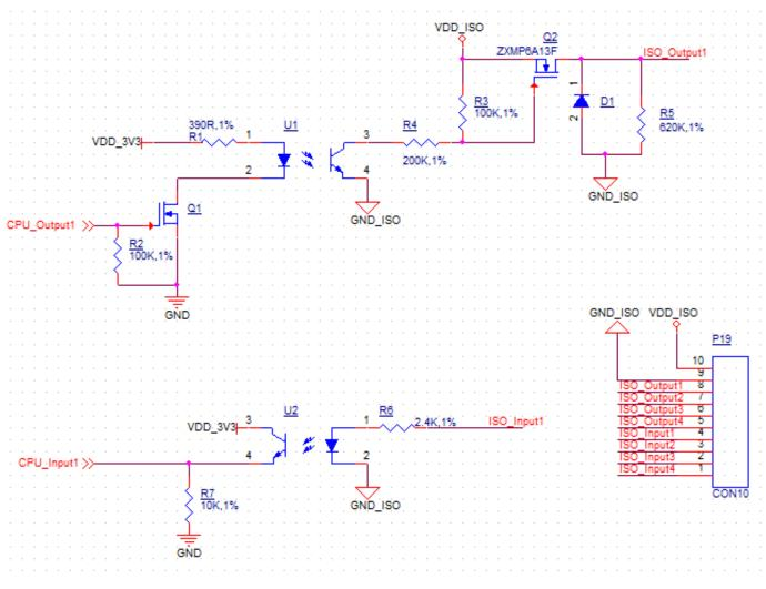
Isolated GPIO reduced schematic
