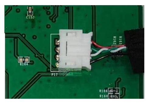
Figure 639: Capacitive Touch Connector
