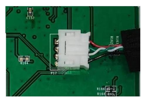
Figure 644: Capacitive Touch Connector
