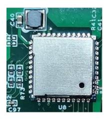
Figure 645: RTL8821CS WiFi/BT Module
