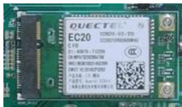
Figure 651: mini-PCle Connector & 4G Module
