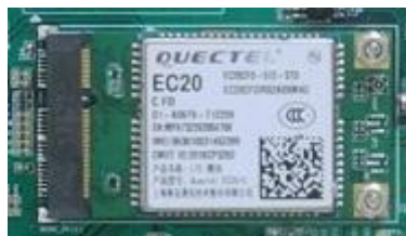
Figure 661: mini-PCle Connector & 4G Module
