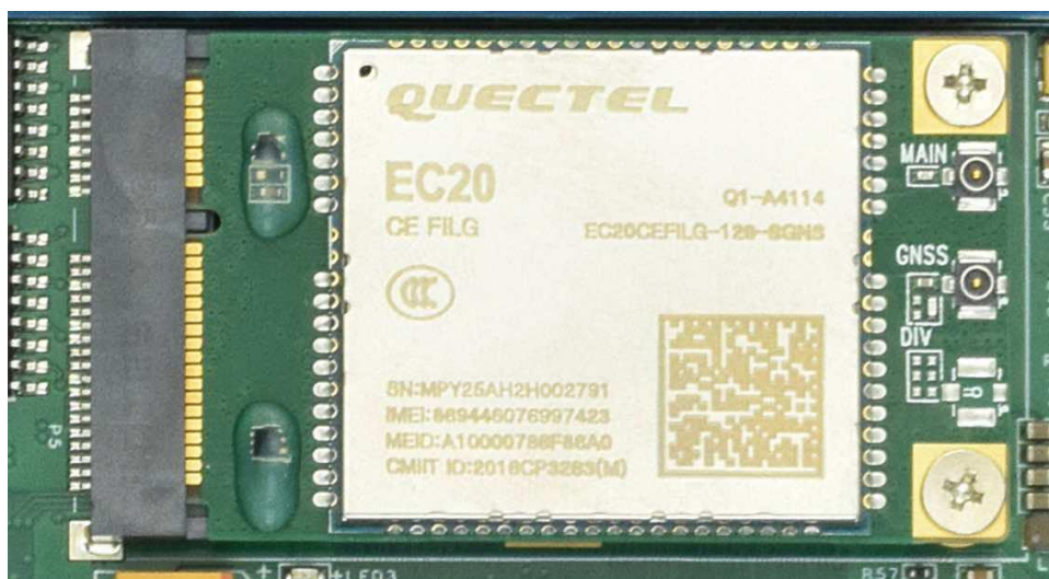
mini-PCle Connector & 4G/LTE Module
