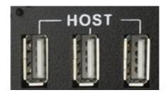
Figure 4: USB HOST Connectors (embedded/enclosed PC version)
