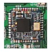
Figure 7: RTL8273 WiFi/BT Module
