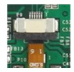
Figure 2: Figure 2: Capacitive Screen Connector
