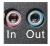
Figure 11: Audio I/O (embedded/enclosed PC version)
