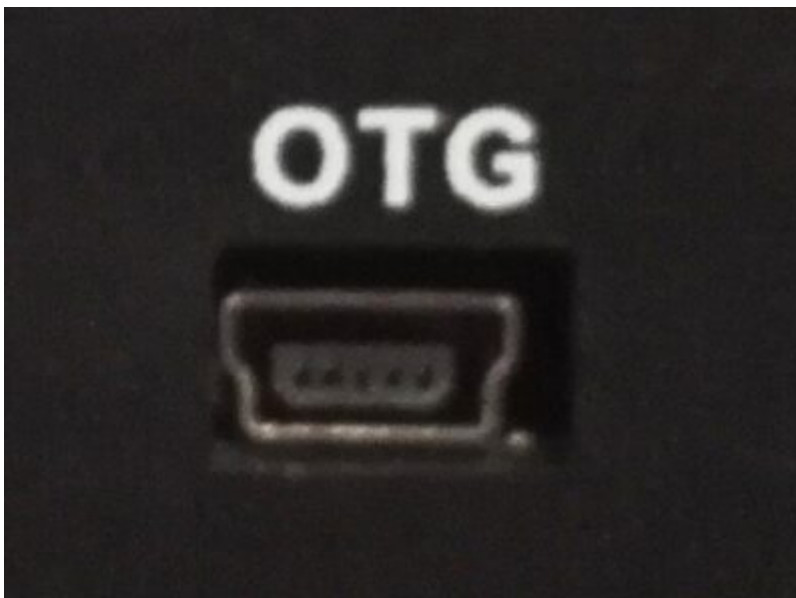
Figure 108: USB OTG Connector
