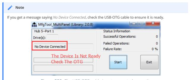
Figure 229: The USB-OTG cable is not connected correctly.
