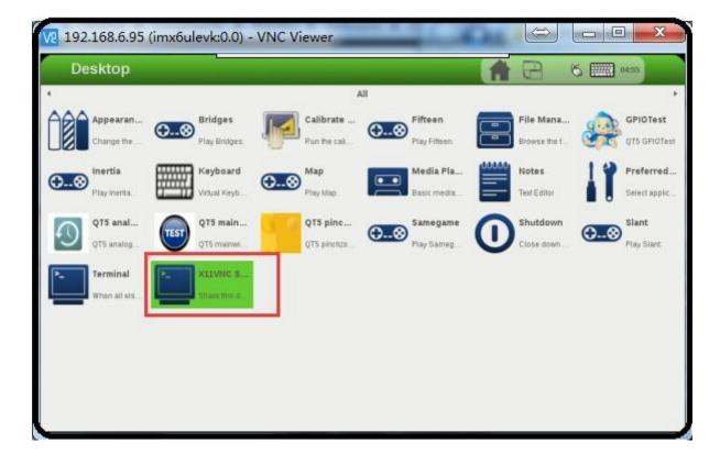
• Use VNC-Viewer in Windows to control it over Ethernet, as shown on the figure below.
