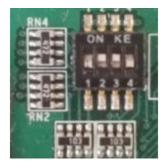
Figure 301: Boot Mode Setup
