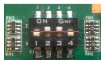
Figure 304: Boot Switch Config
