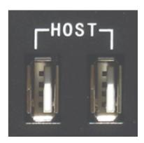
Figure 334: Figure 4: USB Connectors (embedded/enclosed PC version)
