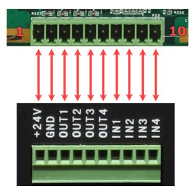
Figure 337: Figure 7: GPIO Terminal (embedded/enclosed PC version)
