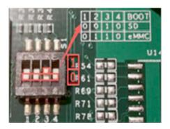
Figure 341: Figure 10: Boot DIP Switch
