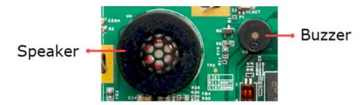
Figure 340: Figure 9a: 2W Micro Speaker and Buzzer
