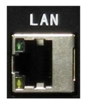
Figure 335: Figure 5: RJ45 LAN Connectors (embedded/enclosed PC version)
