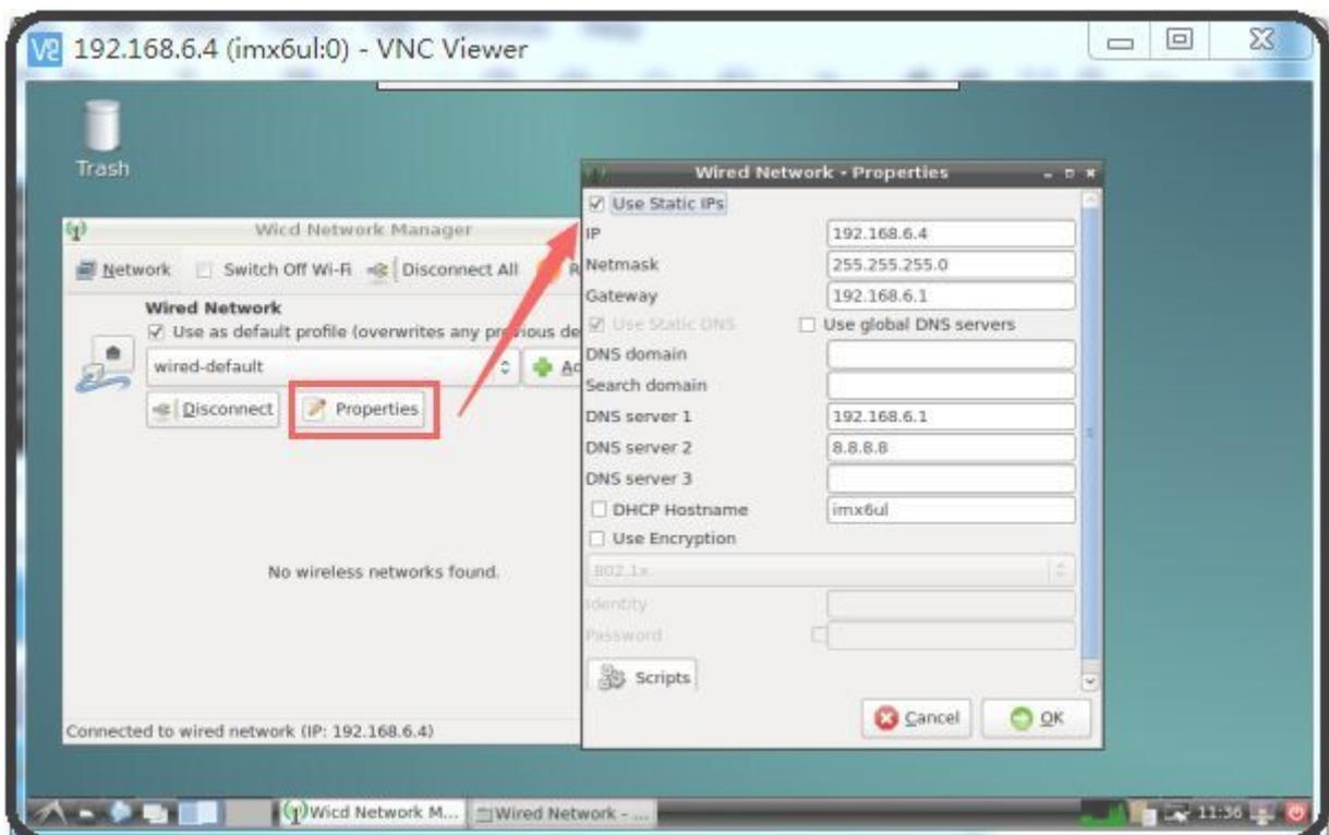
Figure 353: Figure 5a: Setting up Static IP
