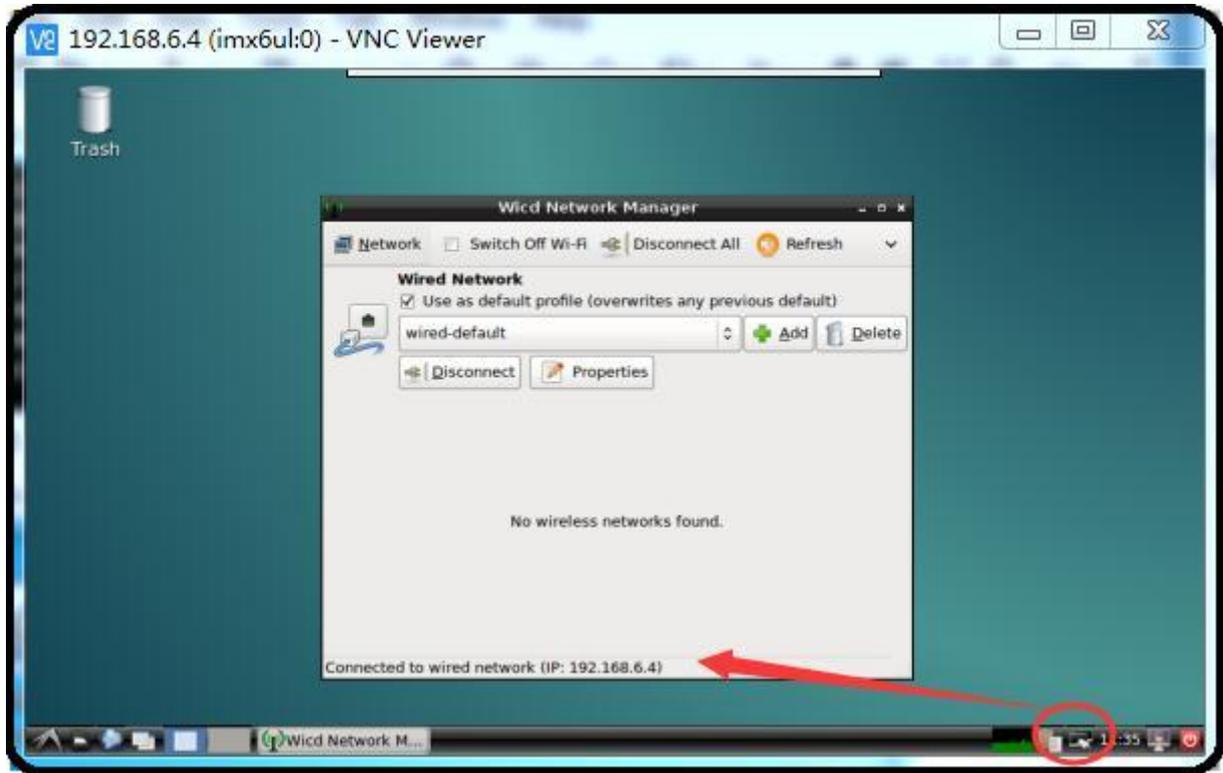
Figure 352: Figure 5: Ethernet Settings (Wired Network Manager)
