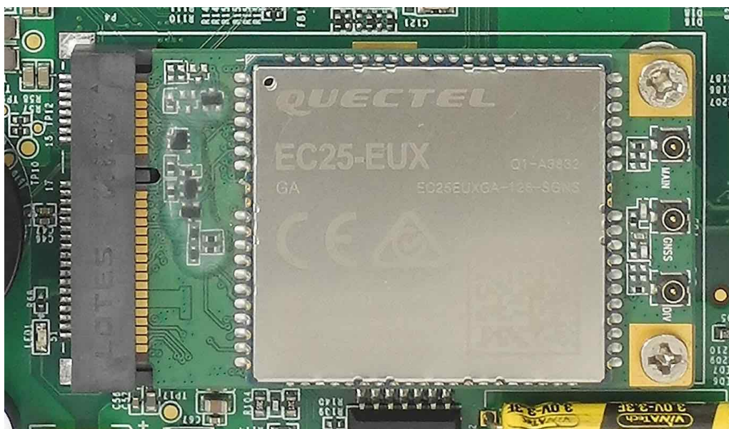
mini-PCle Connector & 4G/LTE Module
