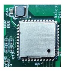
Figure 400: RTL8821CS WiFi/BT Module
