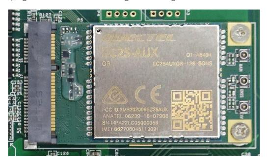
mini-PCIe Connector & 4G/LTE Module
