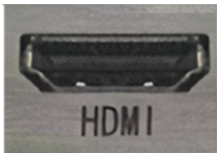
Figure 890: Figure 5: HDMI Connector
