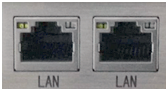
Figure 889: Figure 4: 2 x RJ45 GbE LAN Connectors
