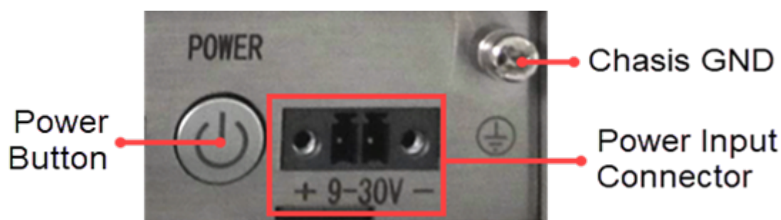
Figure 886: Figure 1: Power Input Section
