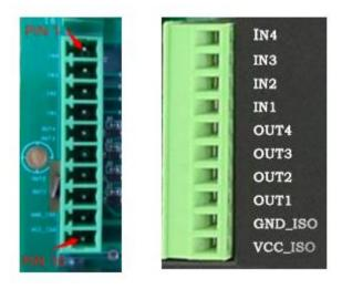
Figure 1040: GPIO Connector
