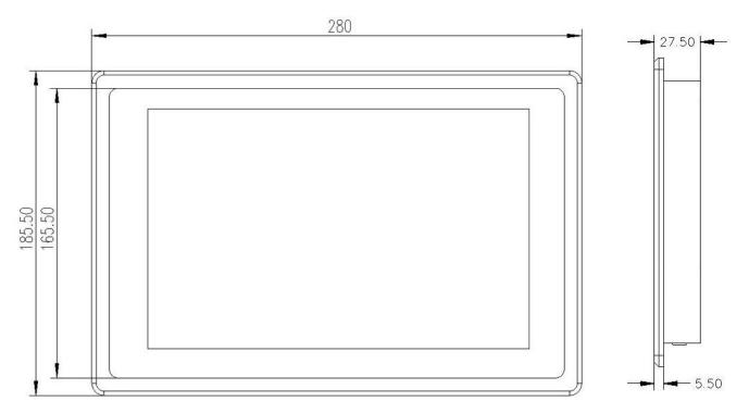
Figure 1054: CS12800RA101P Technical Drawing
