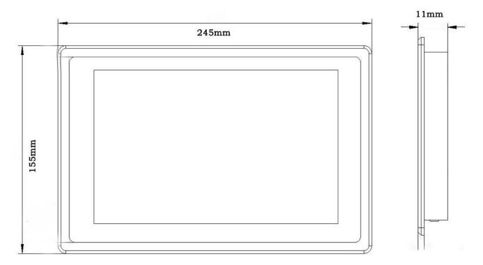
Figure 1053: CS12800RA101E Technical Drawing
