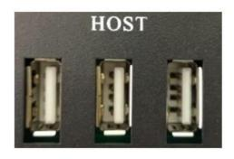
Figure 1041: USB HOST Connectors (embedded/enclosed PC version)
