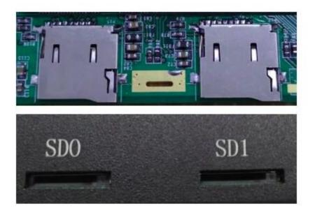
Figure 1048: TF (micro SD) Card Slot
