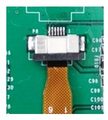
Figure 1038: Capacitive Touch Connector
