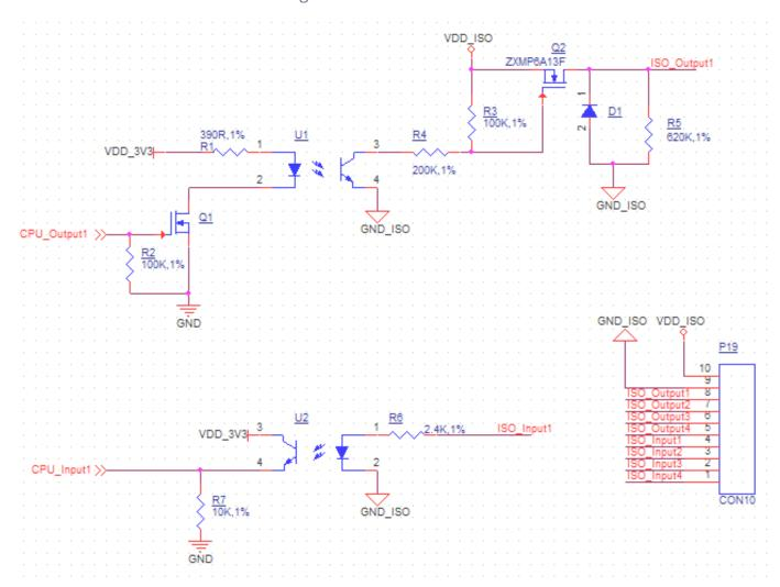
Isolated GPIO reduced schematic
