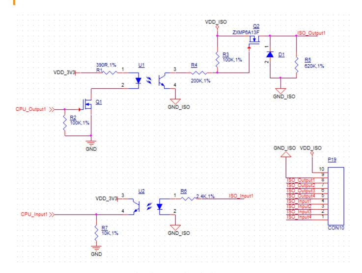
Isolated GPIO reduced schematic
