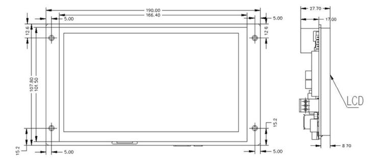
Figure 952: CS10600RA4070E Technical Drawing
