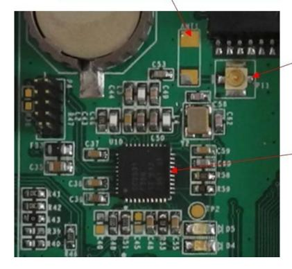
External Zigbee Antenna Connector
