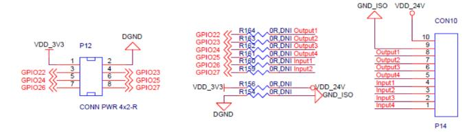
CPU GPIO Reduced Schematic
