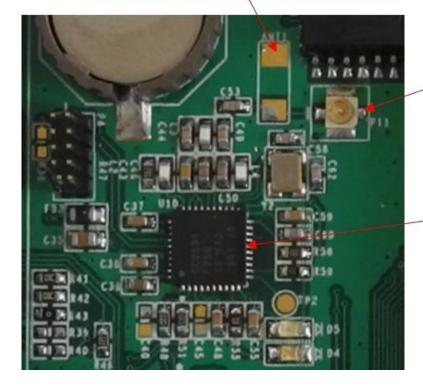
External Zigbee Antenna Connector
