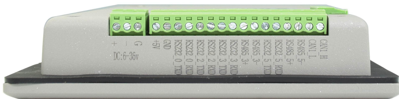
RS232-RS485-CAN on the EPC/PPC-CM5-070 Industrial PC
