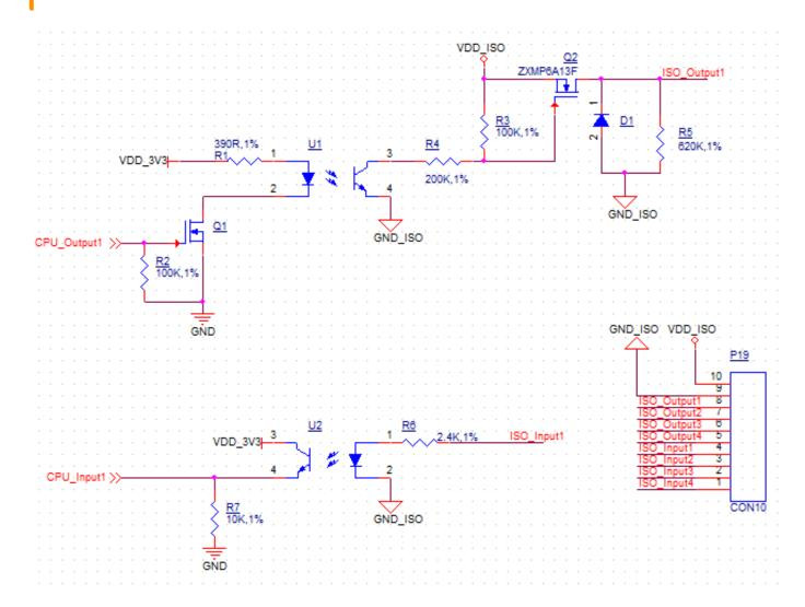
Isolated GPIO reduced schematic
