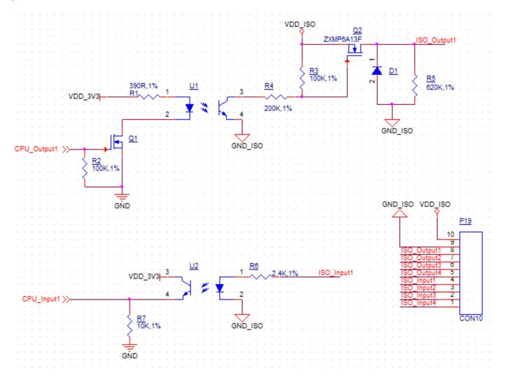
Isolated GPIO reduced schematic
