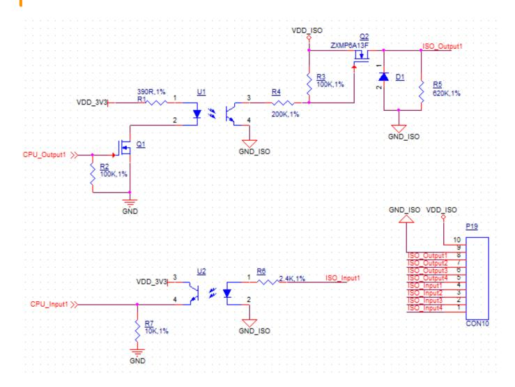
Isolated GPIO reduced schematic
