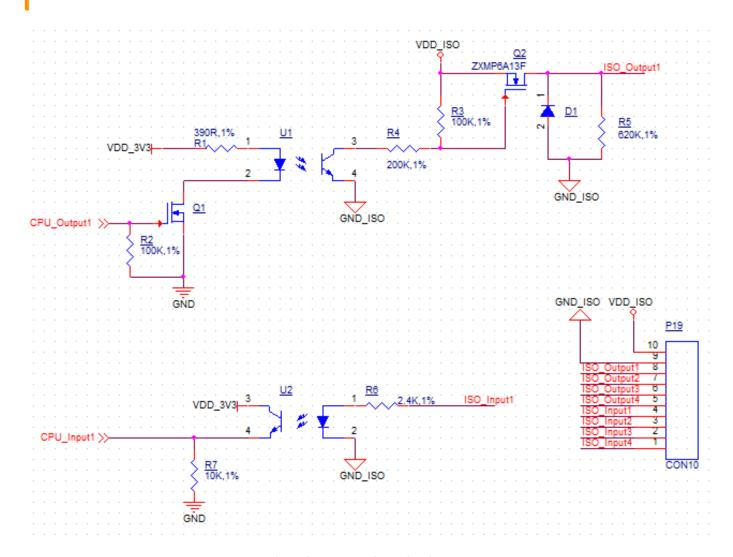
Isolated GPIO reduced schematic
