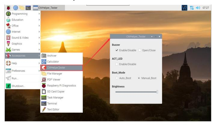
The CMHelper can help customer use keys and onboard buzzer, led, you can use it to control volume, brightness, power, act led, buzzer.
