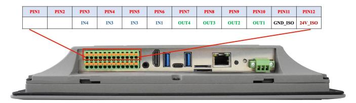
GPIO of PPC-CM5-101 (and above screen size) products
